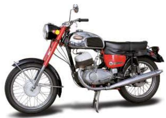
Jawa Californian 350 Years produced: 1967-1974 Engine type: 343cc air-cooled two-stroke parallel twin Claimed power: 28hp @ 5,250rpm Top speed: 69mph Transmission: 4-speed Weight: 337lbs (wet) MPG: 50-70mpg (est.) Price then/now: \$720 (1972)/\$350-\$1,250
